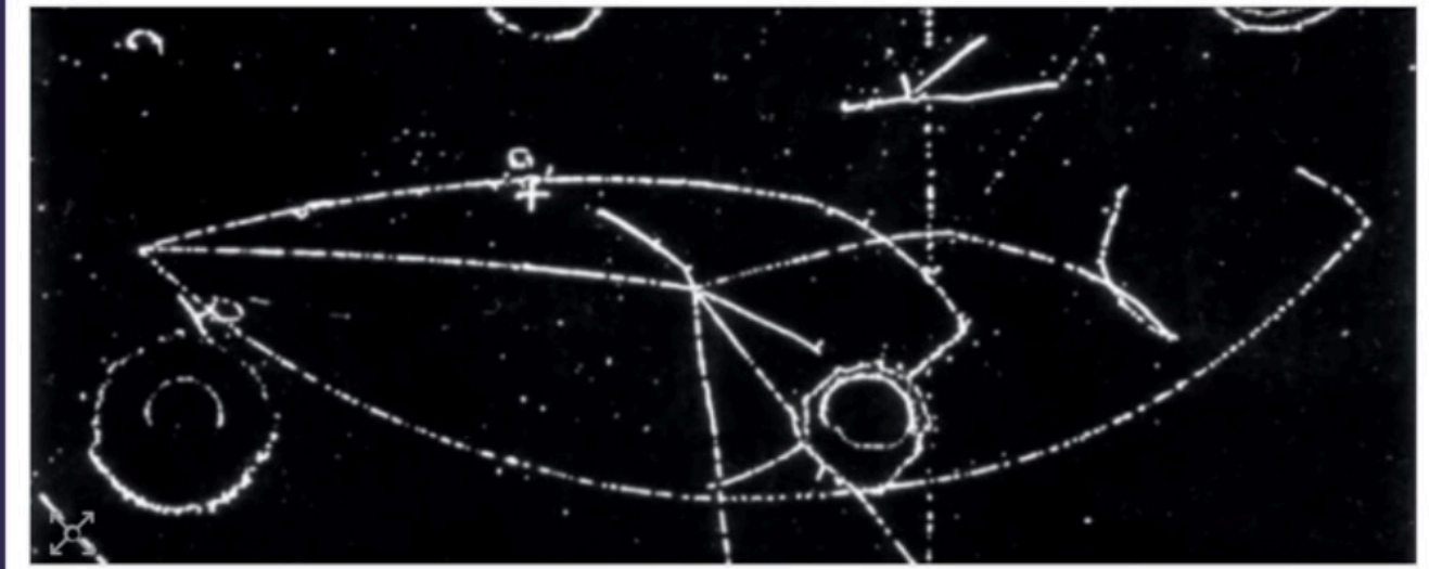
Fig. 1. A hadronic neutral current event, where the interaction of the neutrino from the left produces three secondary particles, all clearly identifiable as hadrons, as they interact with other nuclei in the liquid. There is no charged lepton.
