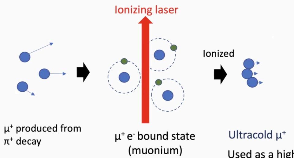
Used as a high-quality  $\mu^+$  beam by accelerating ultracold muons to 300 MeV in g-2 exp.
