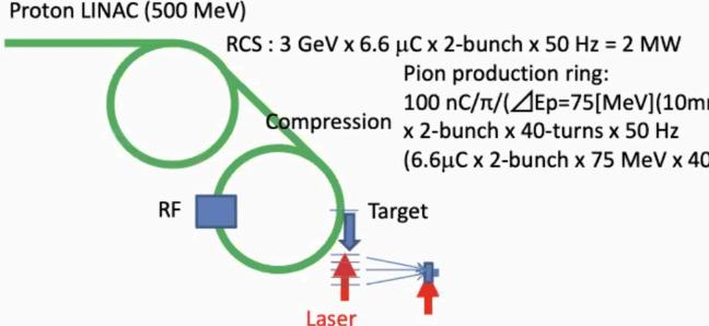
The rate of ultra-cold  $\mu^+$  to  $\pi^+$ : 3.4 % [=  $0.50 \times 0.52 \times 0.60 \times 0.60 \times 0.73 \times 0.50$ ]
