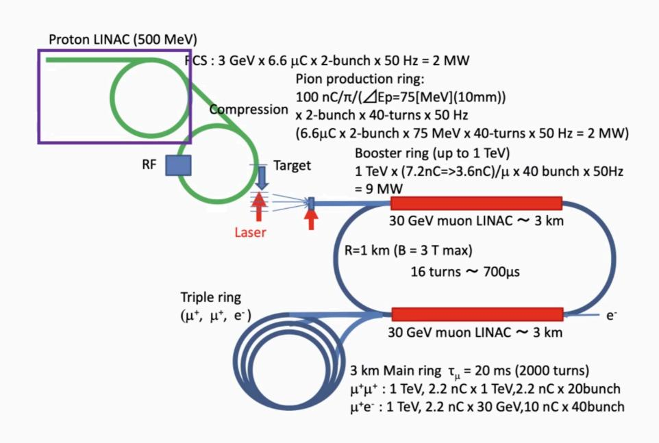
Proton acceleration (Proton LINAC & RCS)  $\longrightarrow$  Pion production (Pion production ring)  $p(3\,\mathrm{GeV}) + C \to \pi^+ + X$
