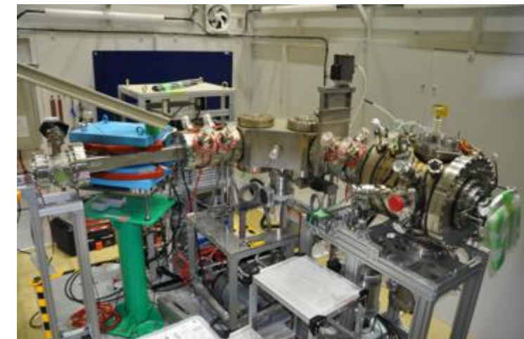
Slow muon beam line constructed for Mu 1S-2S experiment
